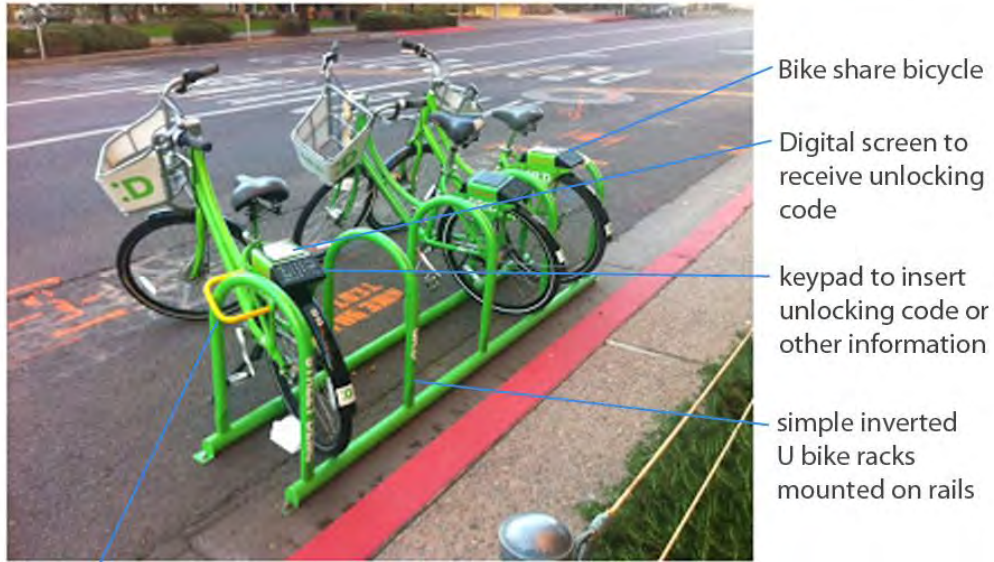
Figure 4: Elements of a 4 th Generation Hub-based, "Smart Lock" Bike Share System
